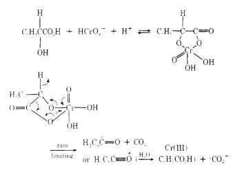
The only known example of a three-electron oxidation of a single molecule is the recently reported oxidation of 2,7dihydroxyheptanoic acid,<sup>2</sup> in which the two reacting centers are separated by a long chain of methylene groups. The chromic acid oxidation of mandelic acid represents the first example of a three-electron oxidation of a molecule in which a C-C and a C-H bond on the same carbon atom are broken simultaneously in the rate-limiting step.
